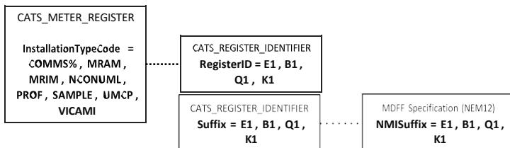
Example of an Interval Meter “Suffix” – Register Level
