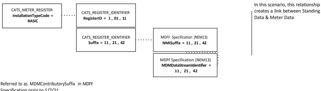
Example of an Interval Meter ‘Suffix’
